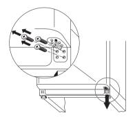
Close the freezer compartment door. Open the fridge compartment door and unscrew the retaining screw for the self-closing mechanism on the top of the freezer compartment door.
